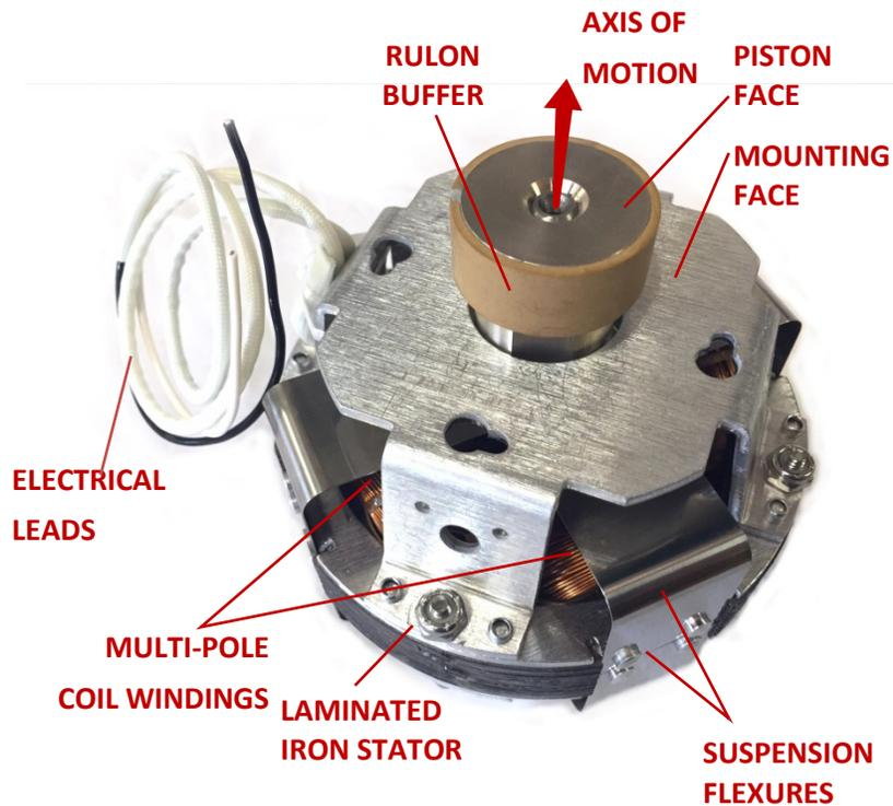
**Figure 1 - Motor Components**
